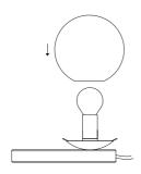
3. Press the clip with hand and install the glass shade
