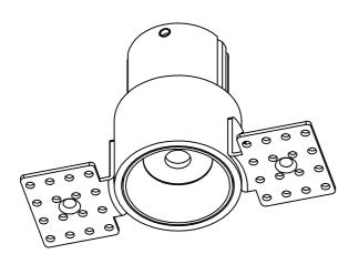
DC439 L104xW44xH64(mm) LED-5W Lamp: CREE COB LED Color: 2700K/3000K/4000K/6000K Color rendering: Ra90 Input: 100V-240V AC Current: Constant 700/500mA Frequency: 50/60Hz Watt: 3W/5WLife span: 50,000hrs Operating temp:  $-20^{\circ}C$  -+40 $^{\circ}C$ IP20 Dimmable: NO
