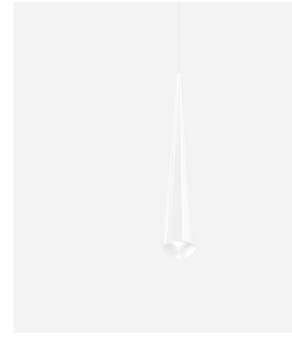
Cone shaped ceiling suspended luminaire made from aluminium; surface White Matt; powder coated; matt texture; RAL 9010; inclusive adjustable cable suspension max. 2200mm in Pure White; PCB 3-step binning; phase-cut dim; light colour 2700 K; binning initial MacAdam  $\leq$ 3 SDCM; CRI  $\geq$  90; 220 - 240 V; degree of protection IP20; Class 1; driver included; light source not replaceable; control gear replaceable by end-user;
