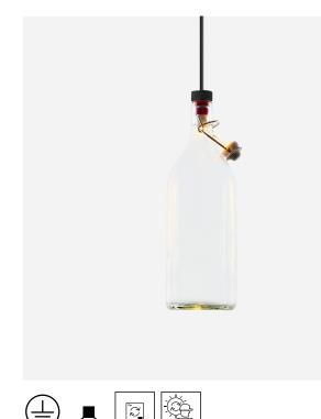
Ceiling suspended luminaire made from aluminium; surface Black Matt; powder coated; matt texture; RAL 9011; PCB 3-step binning; beam angle 34°; light colour 2700 K; binning initial MacAdam  $\leq$  3 SDCM; CRI  $\geq$  80; 100 - 240 V; degree of protection IP20; Class 1; to be combined with a glass bottle; fits bottles inner ø16.5 - 19.5 mm; light source replaceable by Wever & Ducré or by a professional with explicit authorization; control gear replaceable by end-user;
