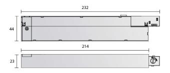
After inserting into the track, rotate the lock counterclockwise to fix the conduction and load bearing fixation!
