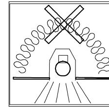
Luminaires not suitable for covering with thermally insulating material.....
