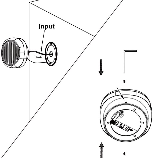
1. Remove the two screws (one upper and one lower)
