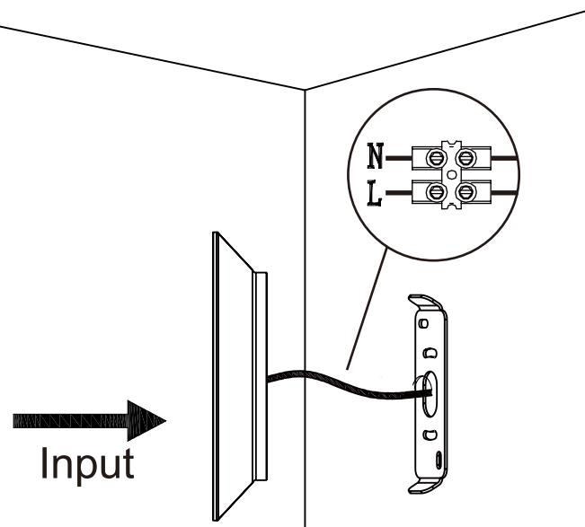
3. Fasten the fixture with screws at the top or bottom
