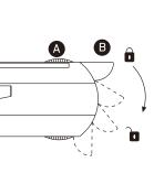
To mount the track adaptor into the track system, first check that the selector knob  $oldsymbol{f A}$  is at OFF position and the adaptor lock **B** is disengaged.
