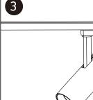
Rotate adaptor lock B clockwise 90° to connect the adaptor to the neutral circuit.
