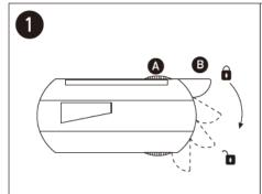
To mount the track adaptor into the track system, first check that the selector knob (A) is at OFF position and the adaptor lock B is disengaged.
