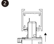
When installing the adaptor into the track, ensure that it is orientated correctly.
