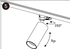
The installation is complete, support can be freely rotated 0° 350° the lamp body can be freely rotated 0° 90°.
