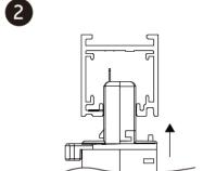
When installing the adaptor into the track, ensure that it is orientated correctly.
