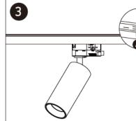
Rotate adaptor lock (B) clockwise 90° to connect the adaptor to the neutral circuit.
