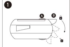
To mount the track adaptor into the track system, first check that the selector knob (A) is at OFF position and the adaptor lock B is disengaged.
