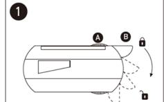
To mount the track adaptor into the track system, first check that the selector knob (A) is at OFF position and the adaptor lock (B) is disengaged.
