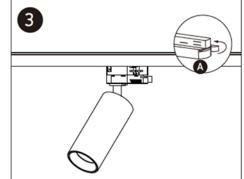
Rotate adaptor lock (B) clockwise 90° to connect the adaptor to the neutral circuit.
