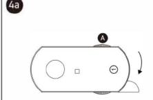
Circuit 1: Rotate the knob (A) 90° clockwise from the starting position OFF, to connect circuit 1.
