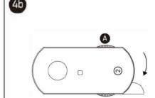
Circuit 2: Rotate the knob @ 90° anti clockwise from the starting position OFF, to connect circuit 2.
