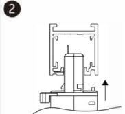
When installing the adaptor into the track, ensure that it is orientated correctly.
