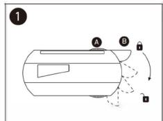
To mount the track adaptor into the track system, first check that the selector knob  ${f A}$  is at OFF position and the adaptor lock (B) is disengaged.
