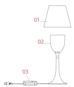
01. transparent diffuser assembly RF625500702. Miss K Table Internal diffuser RF11791
